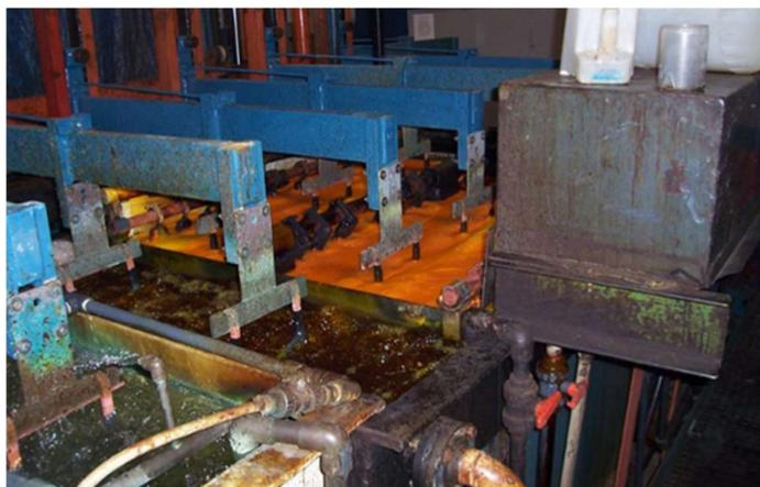
Figure 4: Chromium plating bath (with orange foam) with rinsing baths (EPA, 2009)
